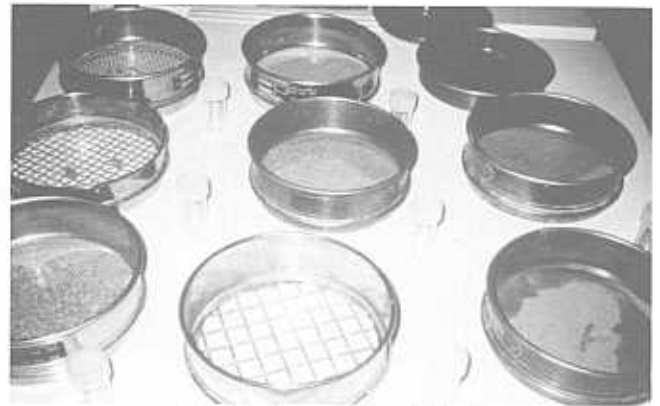
Checking the grain size distribution
