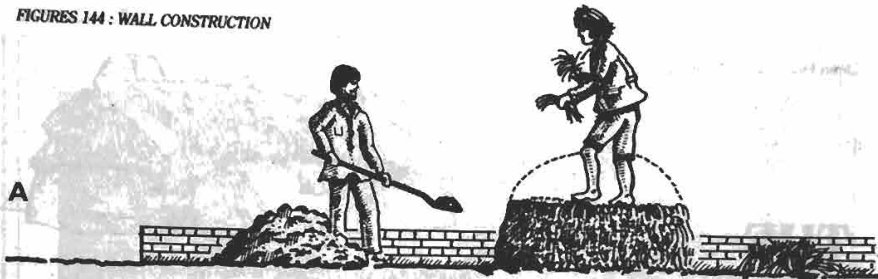
A: PREPARING THE MIX: EARTH AND STRAW
