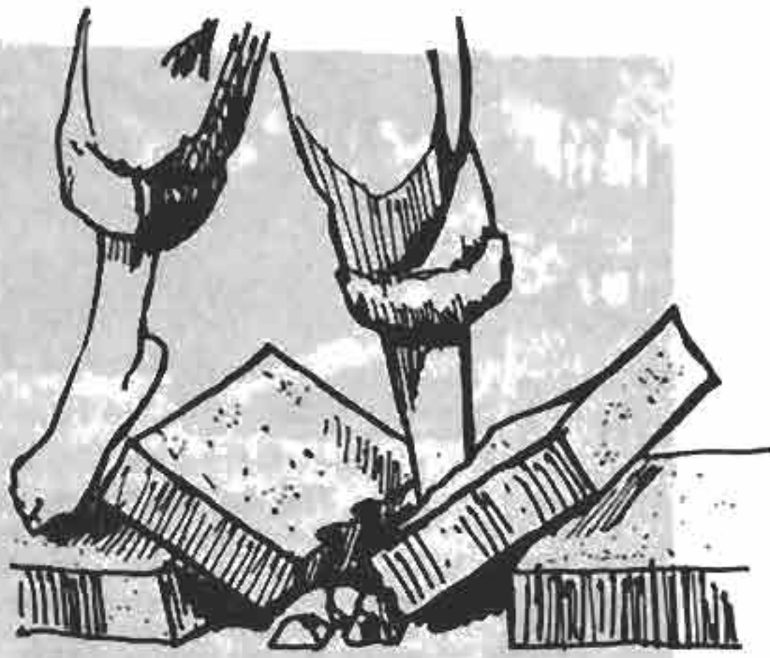
FIGURE 171: BENDING STRENGTH TEST. ONCE DRY THE BLOCKS SHOULD BE CAPABLE OF SUPPORTING A MAN'S WEIGHT FOR ONE MINUTE.
